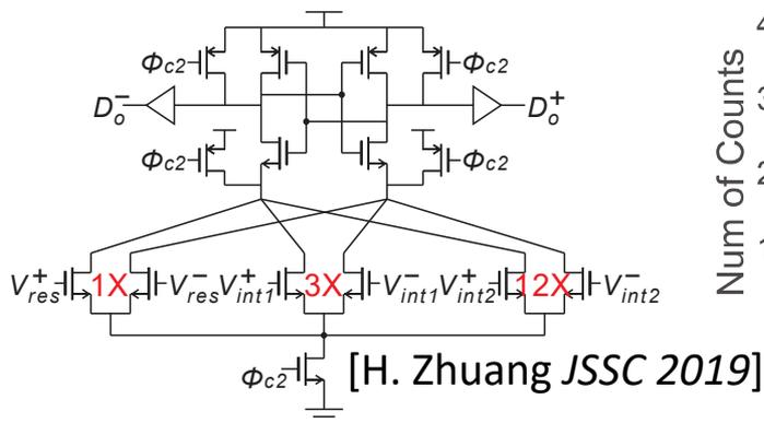
**Source of input pairs separated:**
