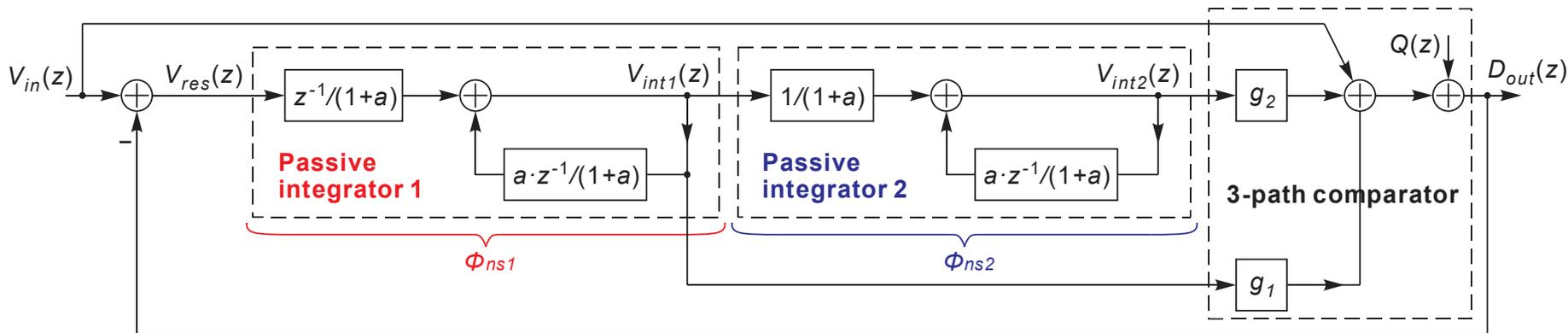
$$D_{out}(z) = V_{in}(z) + \frac{\left(1 - \frac{a}{1+a}z^{-1}\right)^2}{1 + \frac{(1+a)g_1 + g_2 - 2a(1+a)}{(1+a)^2}z^{-1} + \frac{-ag_1 + a^2}{(1+a)^2}z^{-2}} Q(z)$$
