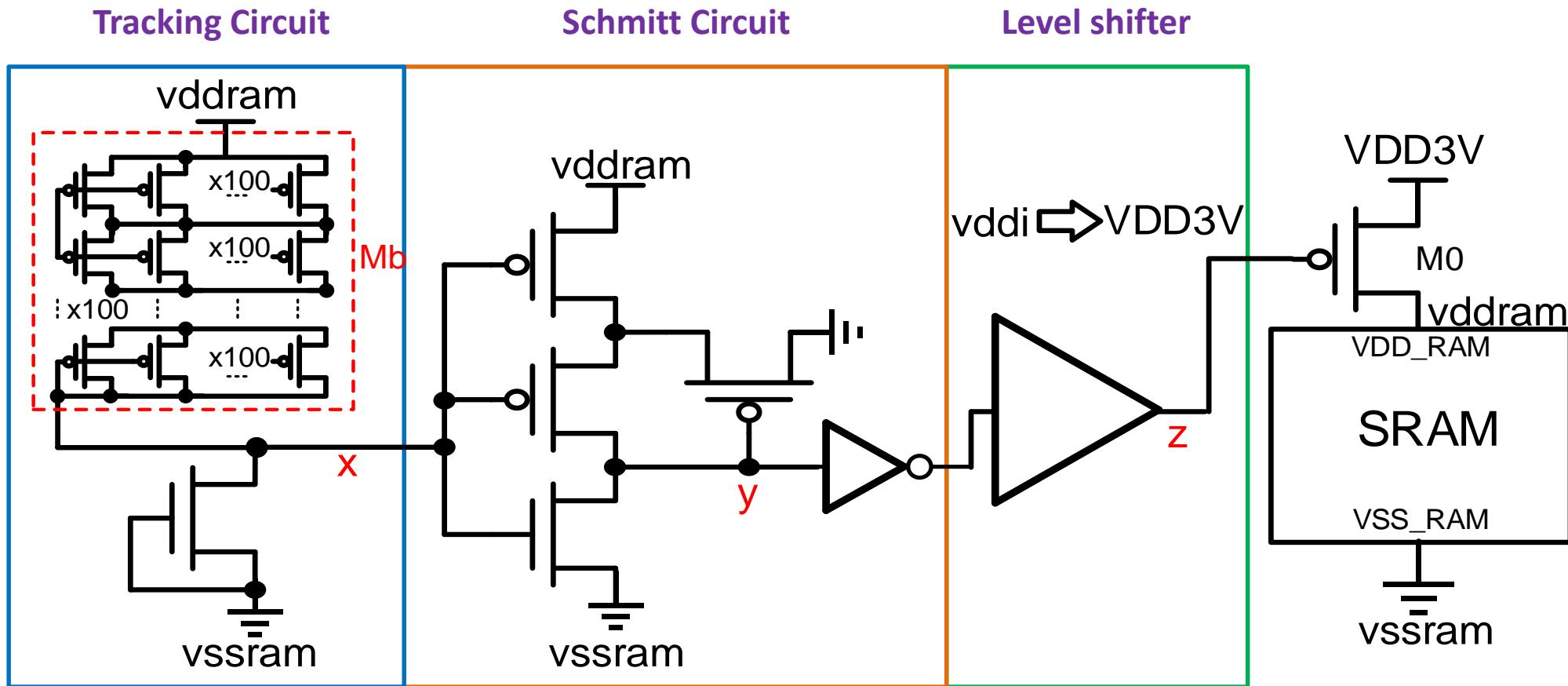
$$\begin{aligned}V_{vddram} - V_{vssram} &= V_M + V_F > V_{DRV} \\&\approx V_M - \frac{kT}{q_p} \ln \left[ 1 - k_1(1 - e^{\frac{-VM}{kT/qn}}) \right]\end{aligned}$$
