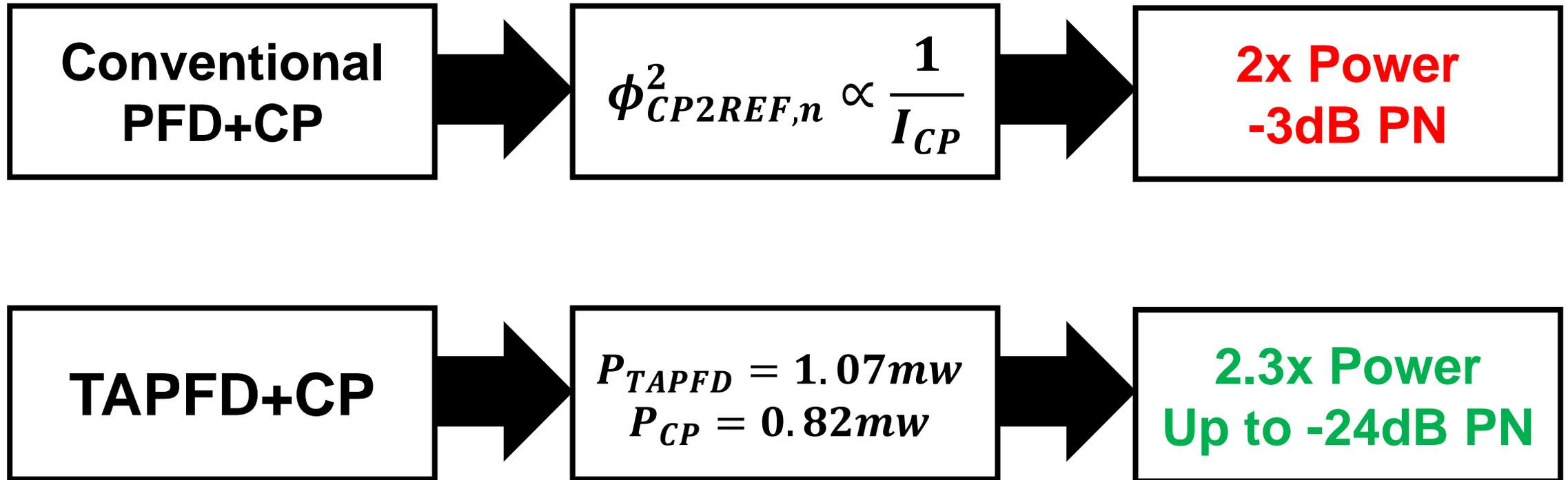
😊 The Power-Noise tradeoff in CP is broken by TAPFD
