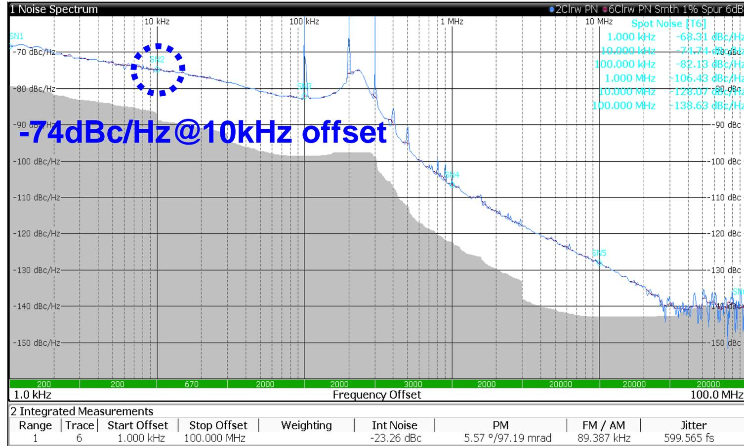
When TAPFD is OFF: in-band noise is dominated by charge pump
