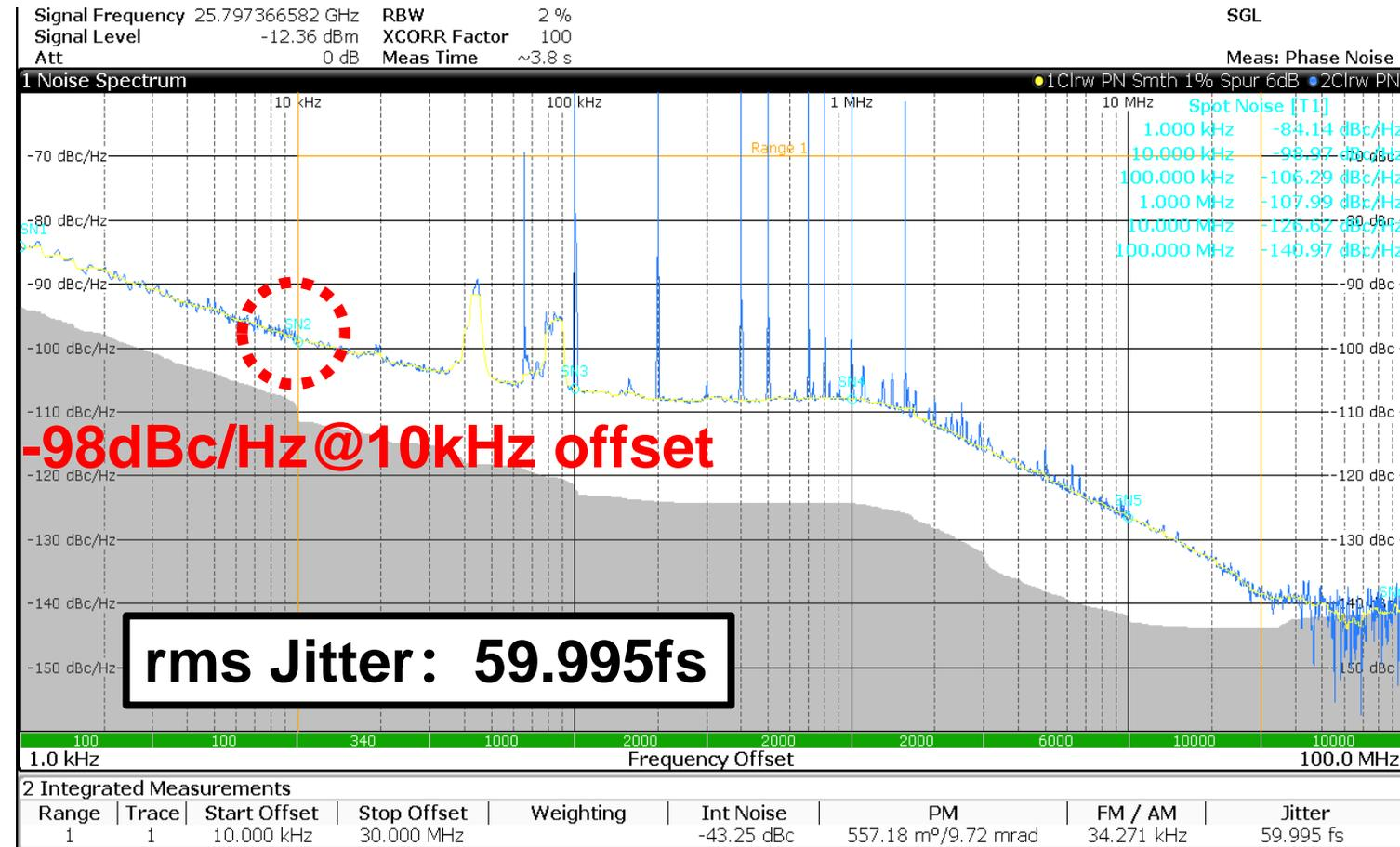
When TAPFD is ON: up to **24dB suppression** of in-band phase noise
