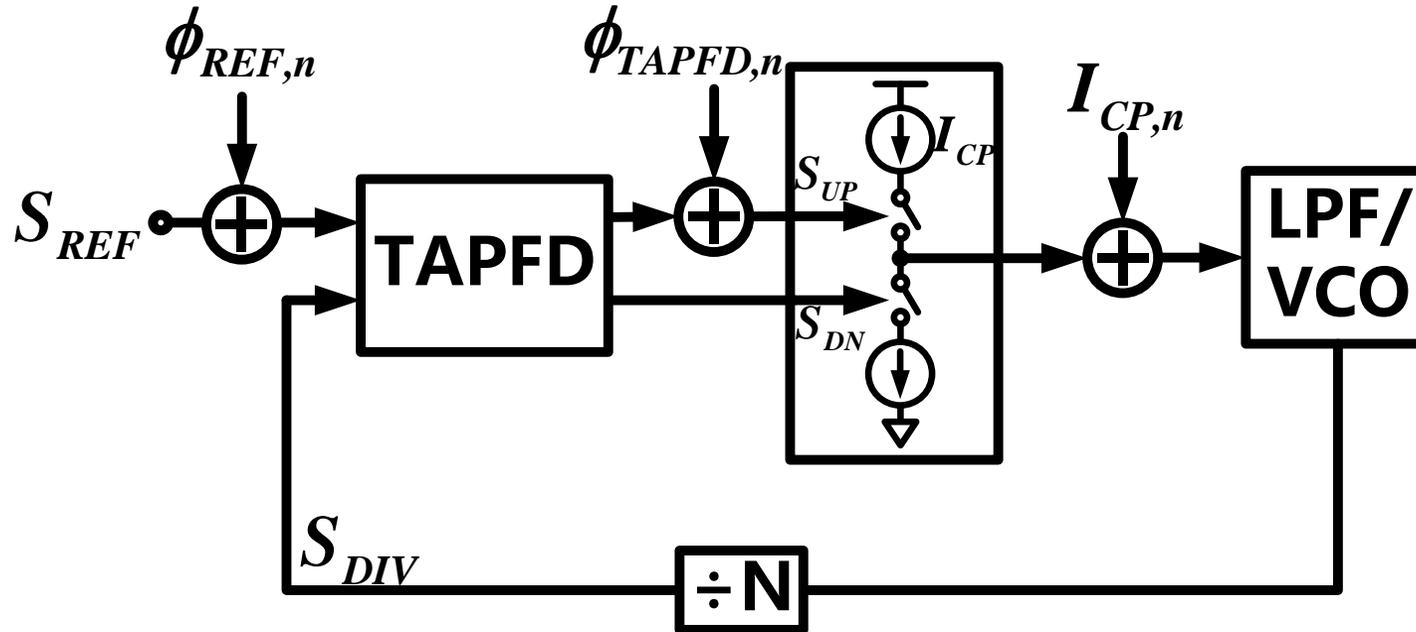
TA-CPPLL Block Diagram with Noise Source
