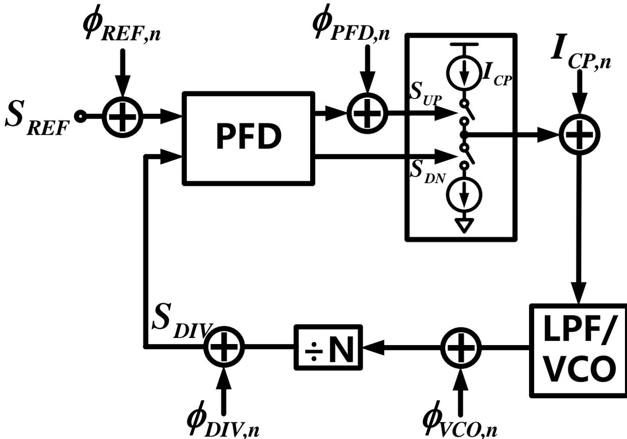
Conventional CPPLL Block Diagram w/ Noise Source
