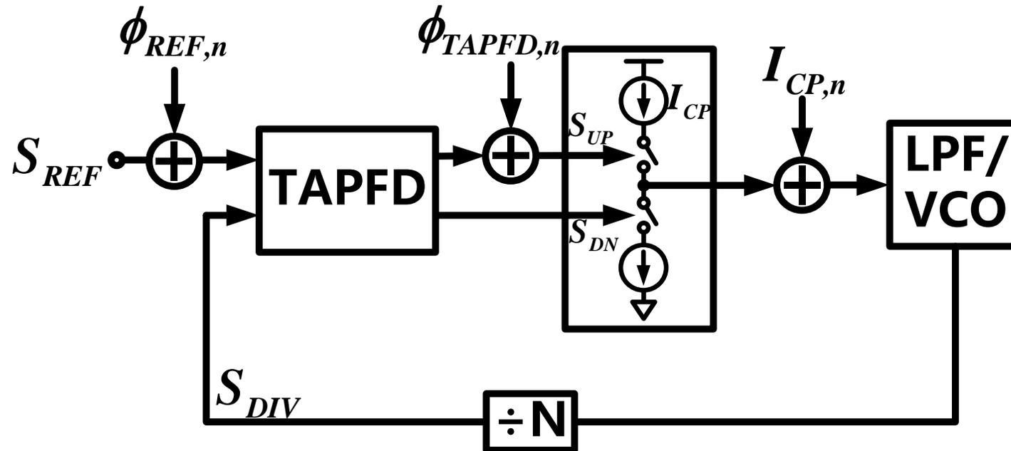
TA-CPPLL Block Diagram with Noise Source
